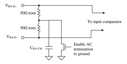
Figure 58. Receiver input termination
