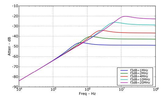
Figure 48. System reference clock jitter rejection
