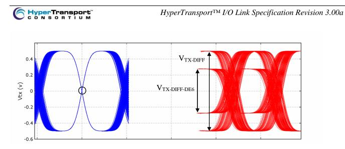
Figure 54. CLK to CAD data eye with some transmit jitter
