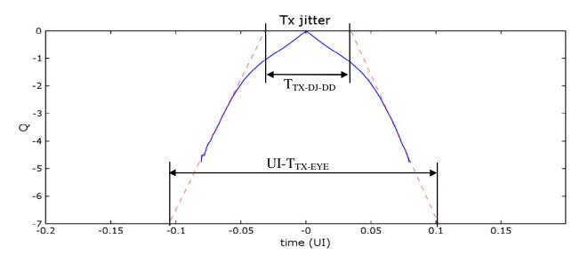
Figure 63. Transmit CAD jitter plotted on Q axis
