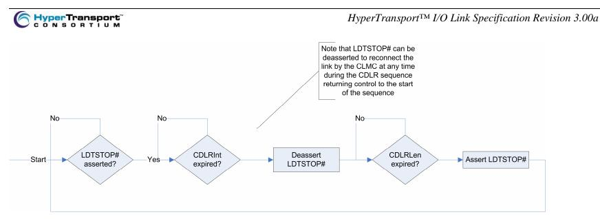
Figure 12. CLMC Sequencing Diagram for CDLR
