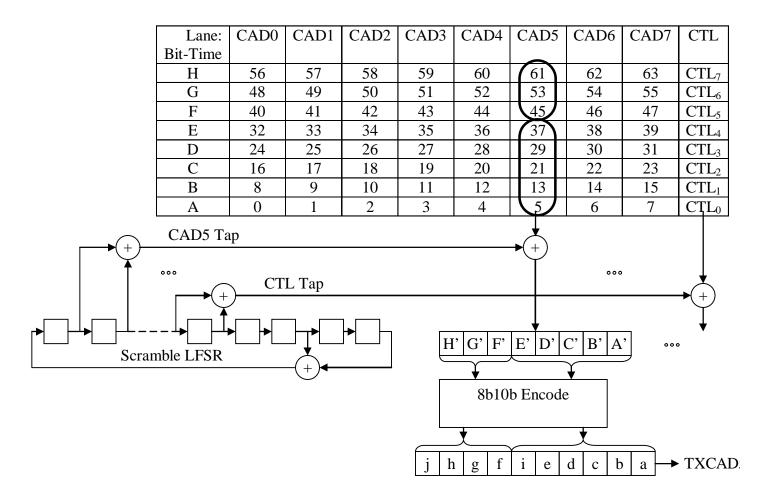
Figure 3. Gen3 Transmitter Order of Operations
