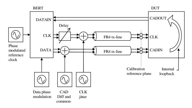
Figure 62. Receiver input compliance test setup
