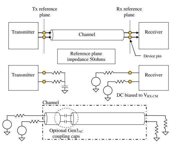
Figure 47. Measurement methodology of HyperTransport<sup>TM</sup> link components
