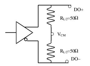
Figure 30. DC Output Reference System Load
