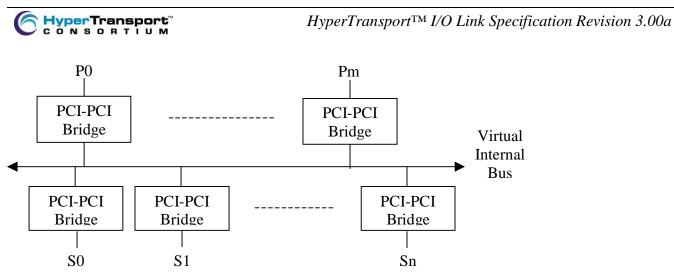
Figure 28. Logical Model of a Switch
