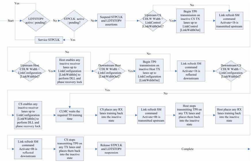
Figure 11. CLMC Sequencing Diagram for CILR
