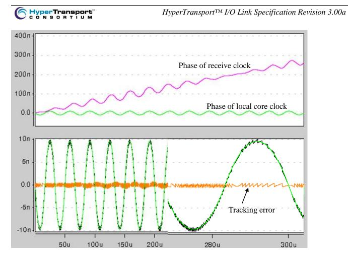
Figure 64. Phase tracking across receiver sync-fifo
