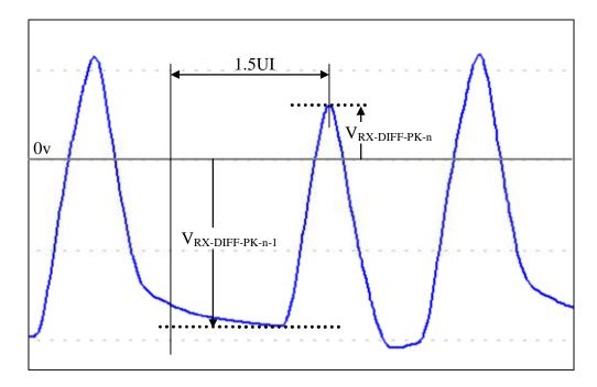
Figure 60. Receiver adjacent bit ratio
