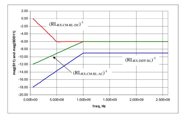
Figure 57. Receiver return loss mask
