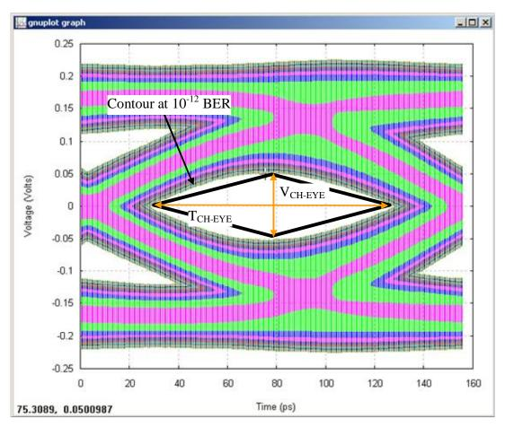
Figure 56. Channel compliance eye diagram
