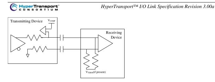
Figure 17. AC Detect Circuit
