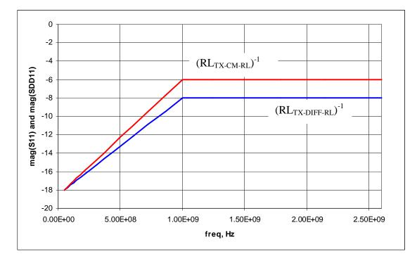
Figure 49. Transmit return loss mask
